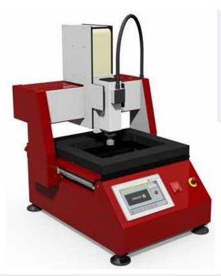
Model for machining where power and precision performance are required. Perfect for engravings and machining of moulds and prototypes. Also with option of vacuum table for the realization of orthopedic templates. Very strong and low maintenance, features of the all FRH series. With transmission by screw&nuts balls recirculation on all axes. Useful working area of 350x250cm and height of 100 mm.
